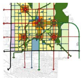
Figure 2-6: Diagram of a street network with greater than 150 intersections per square mile.
